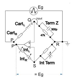
thereby be recovered between point **P'** and point **R**. This is the principle behind the bridge-balance preamplifier.
