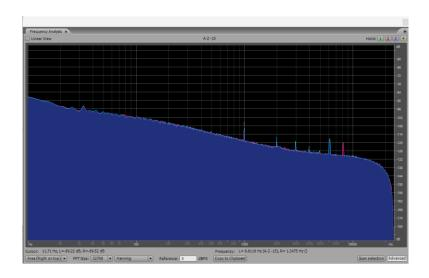
If we filter this with an A-weighting filter, the RMS noise falls to -94dBFS. In the digital domain, this noise is -76dB below standard modulation level, an excellent figure.
