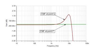
If we arrange *Eg* to be a frequency sweep, we can monitor the voltages versus frequency at point *Q* (the conventional preamplifier input), and at point *P'*. A graph of the results is given. From which, it is very clear how the effect of the interface impedance on the internal impedance of the cartridge is eliminated. Frequency response variation and restriction are both eradicated.
