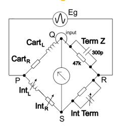
Maxwell's bridge is a development of the Wheatstone bridge, named after James Clerk Maxwell, who first described it in 1873. Maxwell's bridge extends the use of Wheatstone's bridge to measure reactive (not simply resistive) circuit elements. An example is illustrated. This bridge circuit relates directly to the application in which a moving-magnet electrodynamic phono pickup is driving a conventional high-impedance ( $47k\Omega$ ) preamplifier input.
