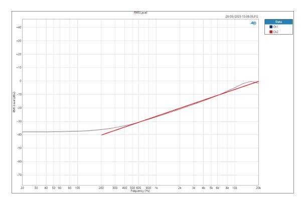
The red line is added and illustrates an ideal 20dB/decade rising response. The frequency response is calibrated in dBu.
